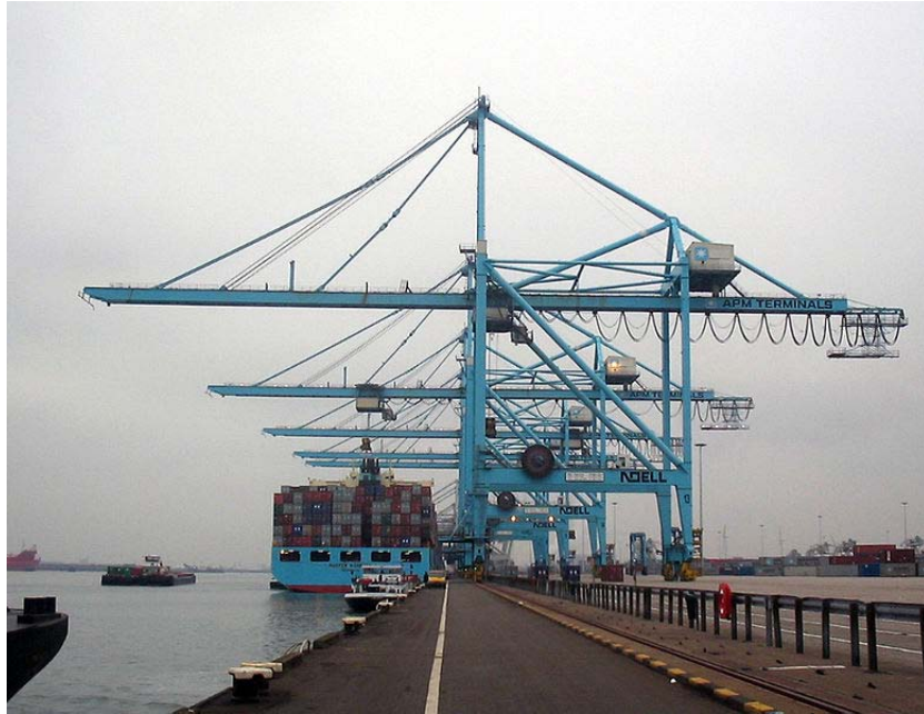
Figure 3. Multiple Gantry cranes loading a ship. 3
